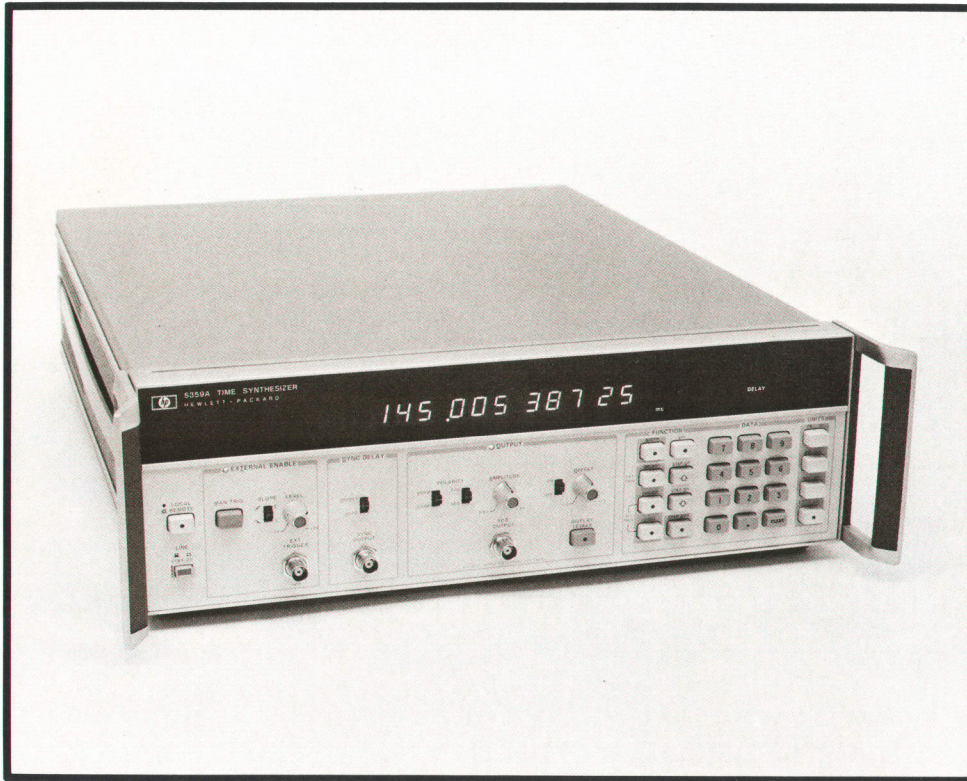
Fig. 2. Model 5359A Time Synthesizer generates precise time delays and pulse widths from 0 to 160 ms (width + delay \leq 160 ms). Absolute accuracy is \pm 1 ns \pm time base error. With the optional high-stability time base, jitter is < 200 ps rms (100 ps typical). Features include keyboard control, HP-IB programmability, and automatic calibration.
